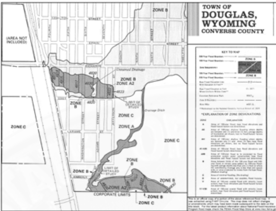
Figure 20. Example of a FIRM for part of the town of Douglas, Wyoming. Zones indicate areas of flooding, inundation, etc. for different events, as described in the text.
