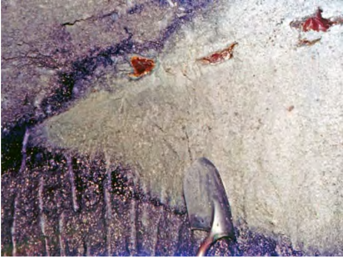
Figure 32. A V-shaped roll exposed in A454. The red and yellow spots in altered ground are clay fragments, which were gray-green before they were altered by mineralizing solutions. The face in the lower half of the photo is water-saturated and light reflecting on the water created the appearance of many small white spots in the black ore. Photo by R. V. Bailey.
