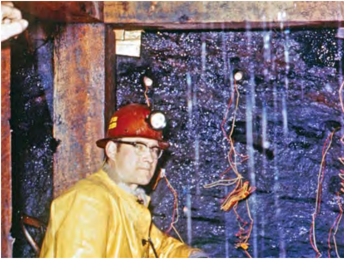
Figure 39. Example of a very good ore face in a very wet stope in A358. Shot holes have been drilled and are being loaded for blasting. The working face was shiny with water and the vertical streaks in the center of the picture were caused by water running into the stope from the back. Photo by R. V. Bailey.
