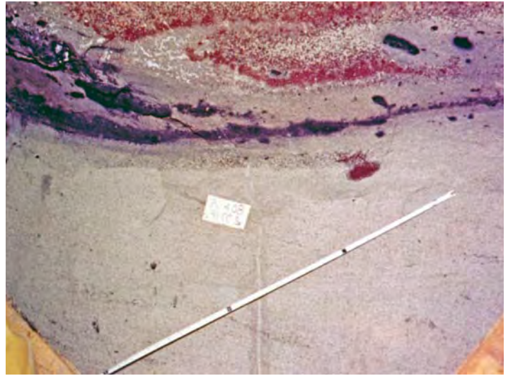
Figure 14. This is a view of the upper limb of the roll seen in Figure 13. Altered ground is in the lower half of the photo. Again uraninite is absent from the tightly-cemented portions of the calcite and is concentrated around plant fragments. The curvature of the contact here may be due to restraint on the advancing solutions by permeability loss in the calcite. In other places calcite also appears to have retarded the advancement of altering-leaching solutions by chemical reaction. Scale: black marks on tape measure are 30.5 cm (12") apart. Photo by R. V. Bailey.
