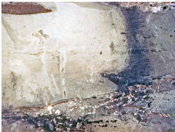
Figure 9. Geochemical front (roll) encountered in A7 Drift a few sets west of A1 Drift. Altered and leached ground is on the left with a band of black high-grade ore along the contact. The white material in the ore is calcite and the red material is hematite within calcite. The altered ground in the left of the photograph is a calcite concretion rich in hematite and which also contains uraninite. Note that the contact freely crosses the cross bedding. Near the center of the photograph, ore protrudes into altered ground at a spot where coalified plant remains are abundant and where there may be less permeability than in the and surrounding sand. Photo by R. V. Bailey.
