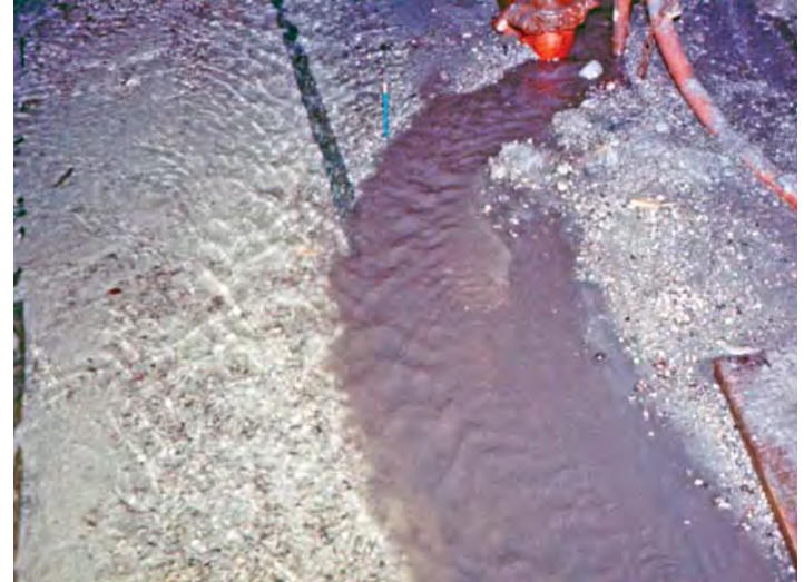
Figure 29. Clear water running down the A9 Drift (toward the camera) is joined by UO_2 -bearing water from a stope where high-grade ore is being mined. A considerable amount of uraninite, which mostly occurs as a sand grain coating is removed from the sand agitation in water in the course of mining. Surface settling ponds were used to recover much of the uranium pumped out in mine waters. Note: the blue pencil in the sand at confluence. Photo by R. V. Bailey.
