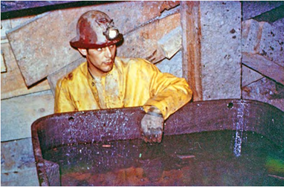
Figure 30. A car containing ore mud is ready to be trammed to the shaft for hoisting to the surface. The fingers of the trammer's glove are in the black glossy mud and his jacket can be seen reflected on the surface of the ore. Much of the Shirley Basin ore shipped to the surface was of this consistency. Behind the trammer, closely-spaced wall lagging can be seen. Photo by R. V. Bailey.
