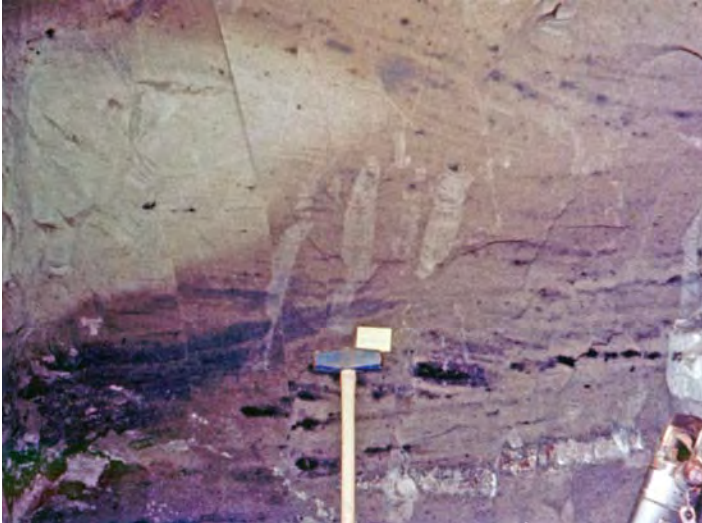
Figure 23. Sage Sand roll south of A7 Drift. This face underground presented an unusual opportunity for the geologist-photographer because an excellent roll was exposed and a large face (about 2.7 m (9') high and 2.1 m (7') wide) was standing open without timber to block the view. The roll here does not display the usual band of rich mineralization along the contact but nevertheless the gradation from barren altered ground on the left to ore on the right is quite sharp. Uraninite is concentrated around plant fragments in the cross bedding. A calcite concretion can be seen in the lower right corner near the pneumatic spader. There is an apparent displacement near the roll due to the sand on the right jutting about one foot toward the camera. Photo by R. V. Bailey.
