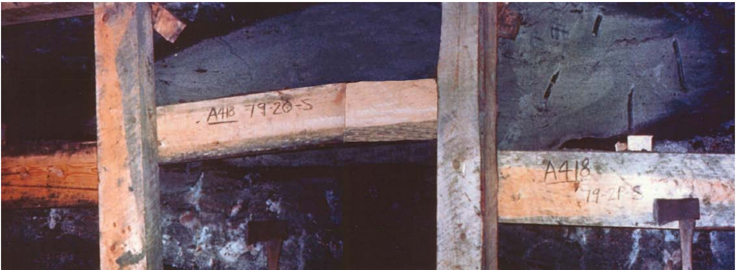
Figure 11. An example of a tongue of altered ground surrounded on all sides by high grade mineralization. This tongue is part of the large body of a altered ground also tongue-shaped, which lies both south of and below this stope (the view in the photograph is toward the south). Calcite is completely absent in altered but is visible as pink to white material in lower part of photo. Vertical marks in altered ground in right-hand of the photo were caused by pneumatic spader. (Note: Two photos were digitally combined to create this image.) Photo by R. V. Bailey.
