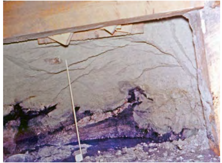
Figure 24. Irregular contact on the lower limb of the Sage Sand roll. Altered ground is above the mineralization. The irregularity is due to restraint on the altering solutions by hematitic calcite and carbonaceous material. Note that the two largest projections into altered ground have a hematitic calcite 'core.' The black fingers into altered ground have a carbonaceous 'core.' This stope was below the water table and two feet of mud and water were in the bottom of the stope when this picture was taken. Photo by R. V. Bailey.
