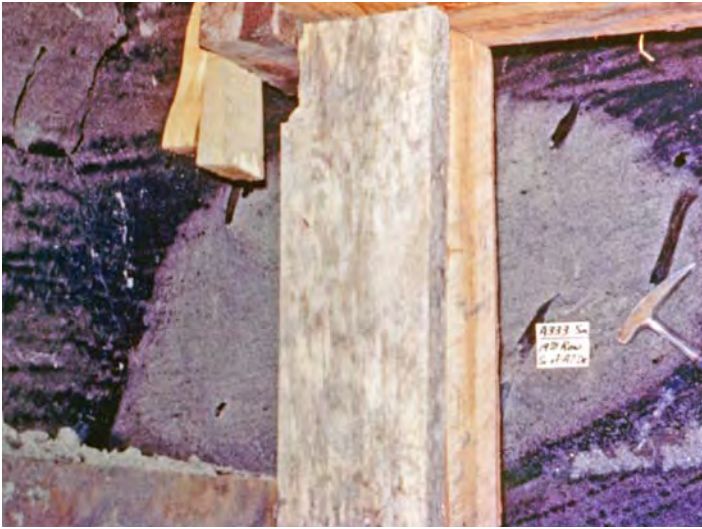
Figure 26. A tube of altered ground surrounded by ore. The angle of the wide part of the tube parallels the dip of the cross bedding. This tube was found in an area of rather complex mineralization where several subsidiary rolls, as well as one major roll were present. The tube was closed on one end, and the other end was connected with the large body of altered ground in the Sage Sand. The calcite in the right-hand corner is shown in more detail in Figure 27 below. Photo by R. V. Bailey.
