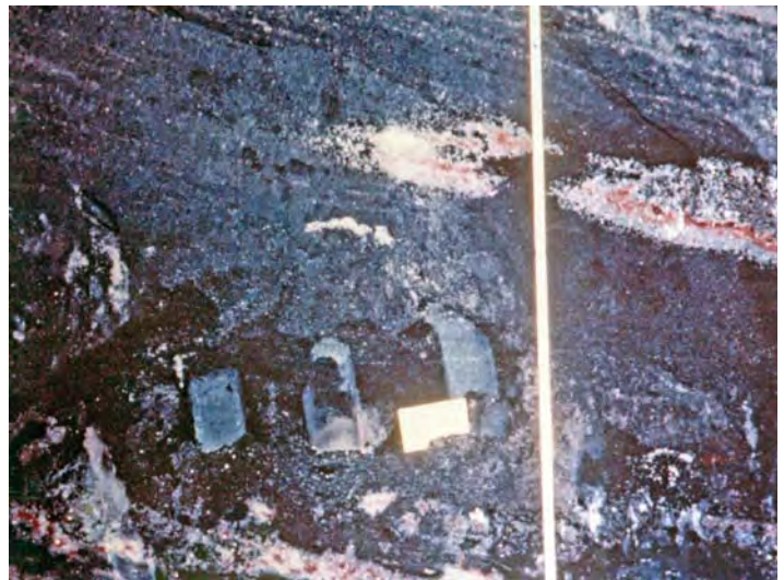
Figure 15. A face of very high-grade ore. No alteration is visible although the photograph was taken just ahead of a roll. The black material is sand, strongly impregnated with uraninite. Hematitic calcite concretions which contain uraninite in the more permeable parts, here were formed parallel to the dip of the cross bedding. The marks in the ore near the card were made by a pneumatic spader. Scale: yellow card is 10 cm x 15 cm (4" x 6"). Photo by R. V. Bailey.
