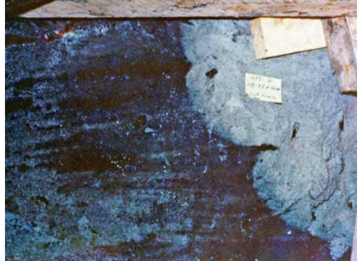
Figure 25. Black high-grade ore is here concentrated along the contact. Cross bedding which is invisible in the altered ground is easily recognized in the ore. Timbering and lagging very often prevented photographing interesting faces seen in the mine. Photo by R. V. Bailey.
