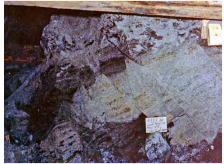
Figure 28. A roll with distinctly rusty altered ground on the right. The inclination of the roll with the cross bedding is strictly a local feature. The gray sand just above the altered ground is unaltered ground, which has fallen down from above. The cavity and timber in the upper left corner indicates that the set above the photo has been mined out. Photo by R. V. Bailey.
