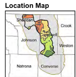
Figure 11. Spatial distribution of TDS for produced water from the Upper Wyodak coal zone within the core producing area. Note increase in TDS from southeast to northwest.
