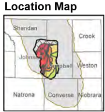
Figure 8. Spatial distribution of TDS for produced water from the Wyodak Rider coal zone within the core producing area. Note increase in TDS from southeast to northwest.
