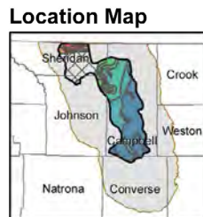
Figure 12. Spatial distribution of SAR for produced water from the Upper Wyodak coal zone within the core producing area. Note increase in SAR from southeast to northwest.
