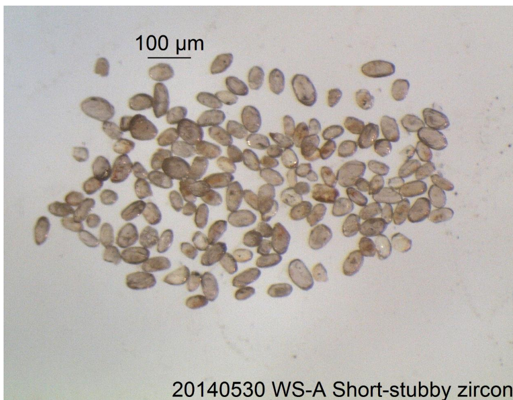
Figure 2. Examples of short and stubby zircons isolated from Antler granite sample. This subpopulation had the highest survival rate from the first step of dissolution (10%). All the CA-
