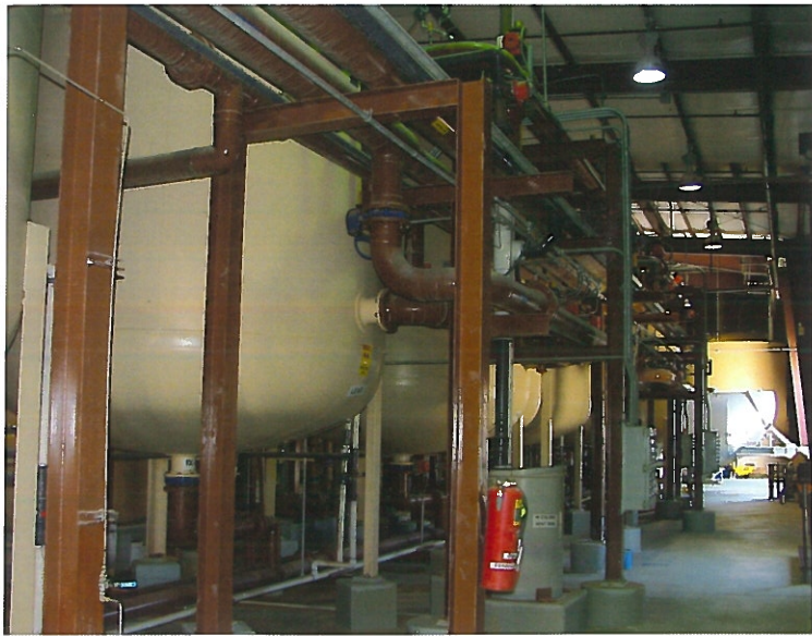
Figure 2. To process uranium into yellowcake, large ion exchange columns are used to concentrate uranium-bearing compounds onto resin beads.
