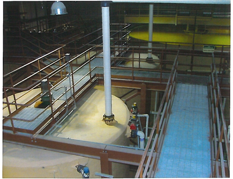
Figure 3. Various tanks are used in the yellowcake production process, including for water storage and the elution and precipitation processes.
