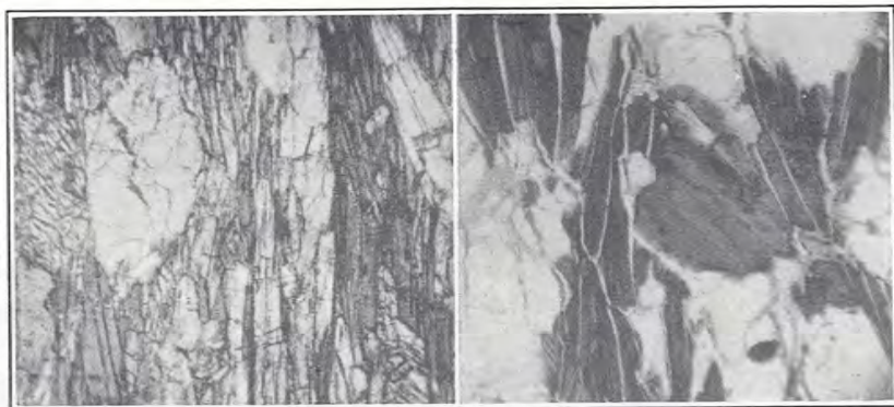
(2) Biotite altering to vermiculite in granite. \times 135 .
