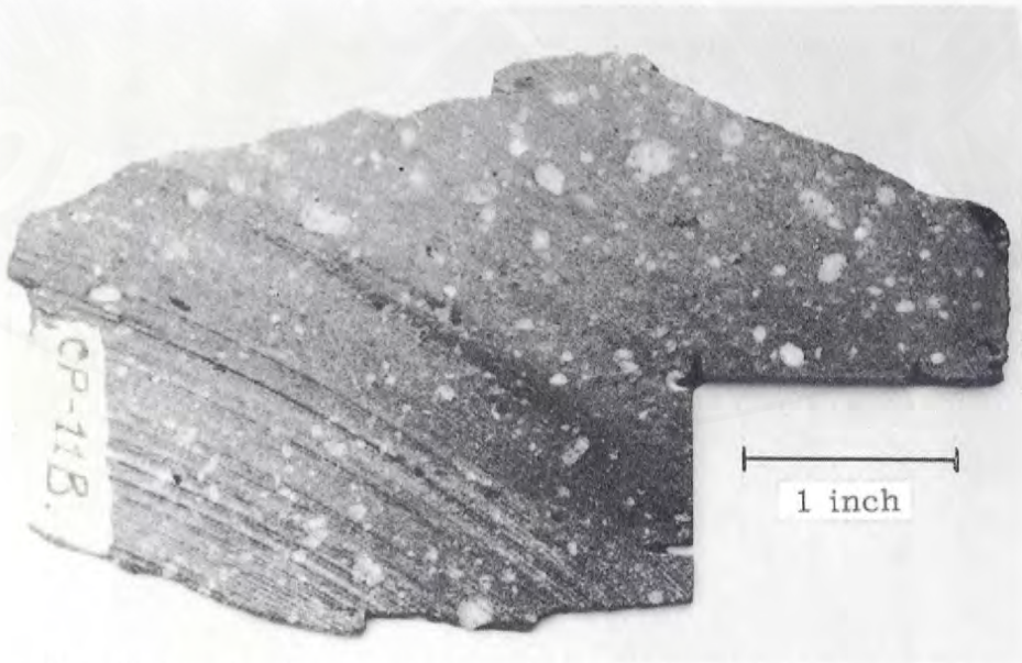
Pl. 4, B. Sawed surface of metagglomerate from locality 1-3. Insets are quartz, feldspar, hornblende, and biotite.
