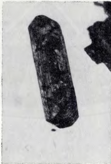
C. Photomicrograph of malacon zircon from the Sanostee, N. Mex., deposit, showing zoning and fracturing. Ordinary light x 155.
