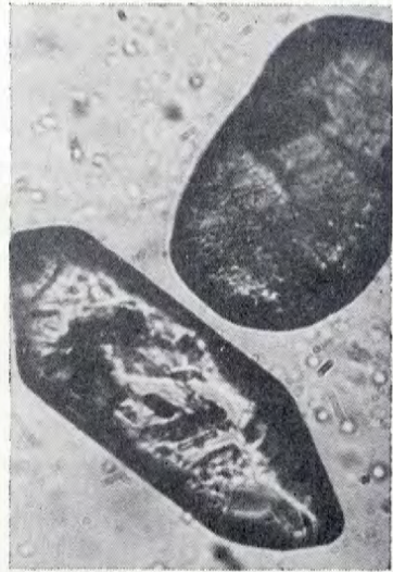
B. Photomicrograph of euhedral colorless and well-rounded reddish-violet zircon from the Grass Creek deposit. Ordinary light x 200.
