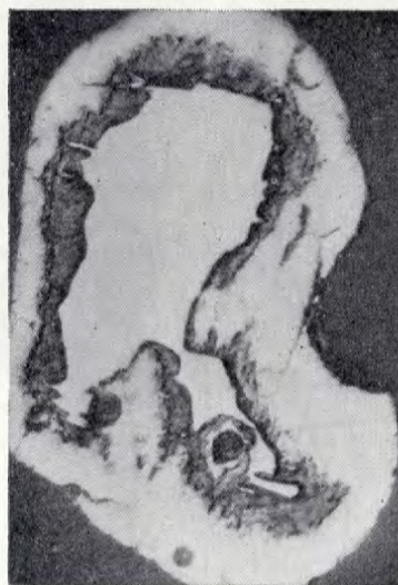
C. Photomicrograph of highly altered ferrian ilmenite(?) from the Grass Creek deposit. Separated at 0.20 ampere. Ordinary light x 405.
