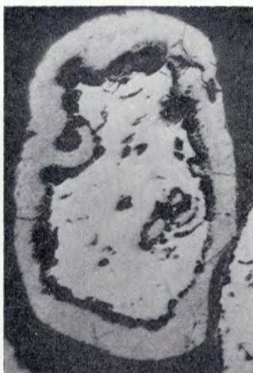
B. Photomicrograph of ferrian ilmenite (?) from the Grass Creek deposit (showing well-developed alteration rims. Separated at 0.10 ampere. Ordinary light x 405.
