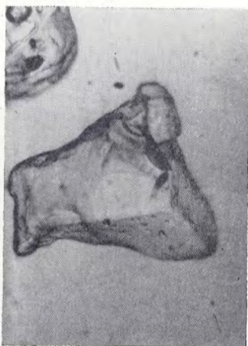
B. Photomicrograph of irregular-shaped pyralspite garnet from the Poison Spider deposit showing facets and pits. Ordinary light x 205.
