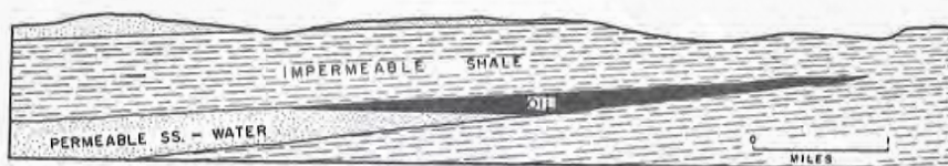
FIG. 36. Cross section of a stratigraphic trap for hydrocarbons.
