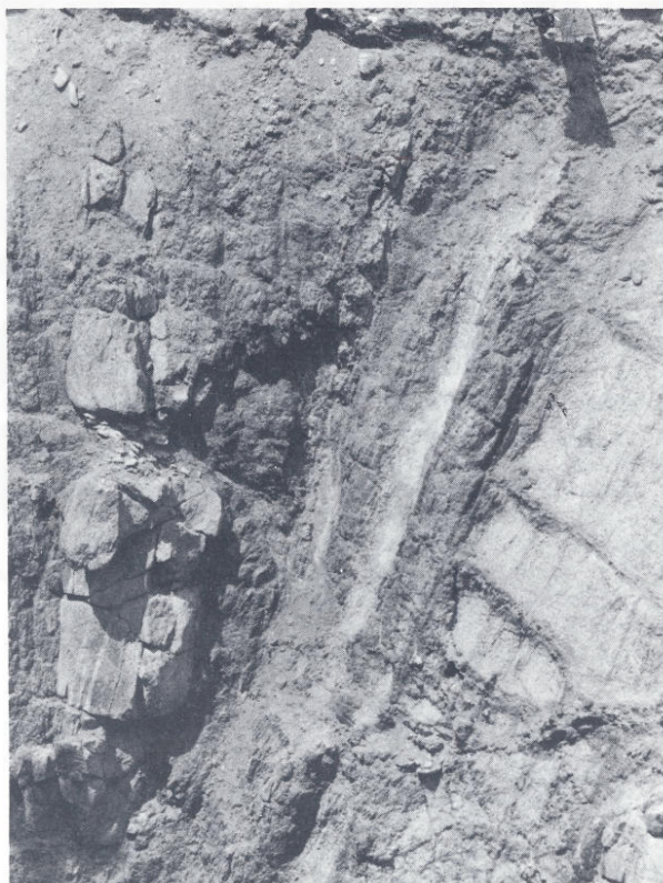
PHOTO 13. Fault zone at the Louise Mine (SE \frac{1}{4} Sec. 35); illustrates the nature of the Comstock-type, clay-rich, fault group. Scale is provided by 6" x 6" mine timber in upper right.
