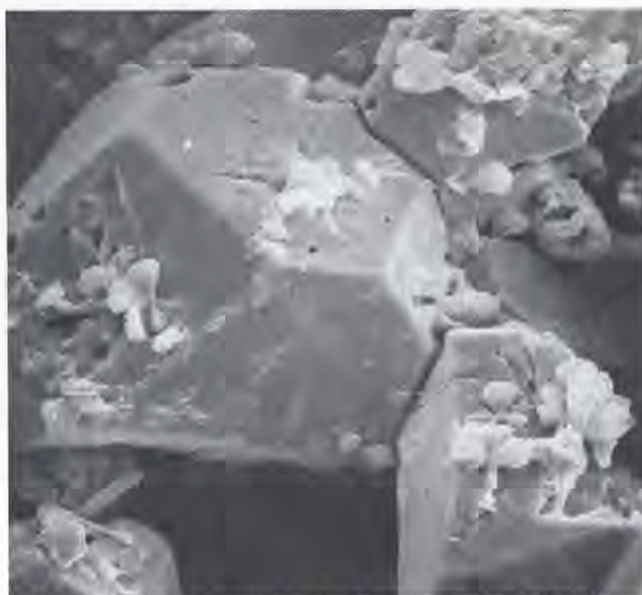
FIGURE 1. Pyritohedrons of pyrite (FeS 2 ) with a later Va mineral in sheaf-like aggregates on the crystal faces (750x). Lower Eocene, Shirley Basin, Wyoming.
