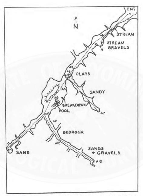
FIGURE 21 — A cave survey notebook, illustrating two facing pages. The data page lists, across the top, distance, compass direction or aximuth, inclination, distance to the left, right, floor and ceiling, and passage cross-sections. The sketch page contains a carefully drawn representation of the cave passage and features, indicating their relation to survey points and lines.
