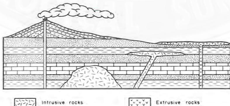
FIGURE 18—Cross-section illustrating the relationship between intrusive and extrusive igneous rocks and bedded sedimentary rocks
