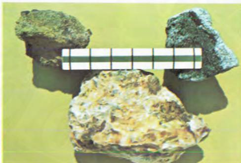
PLATE V-3 Oxidized (yellow) and unoxidized (black) uranium minerals from Wyoming (Specimens courtesy of James M. Hunter, Casper)
