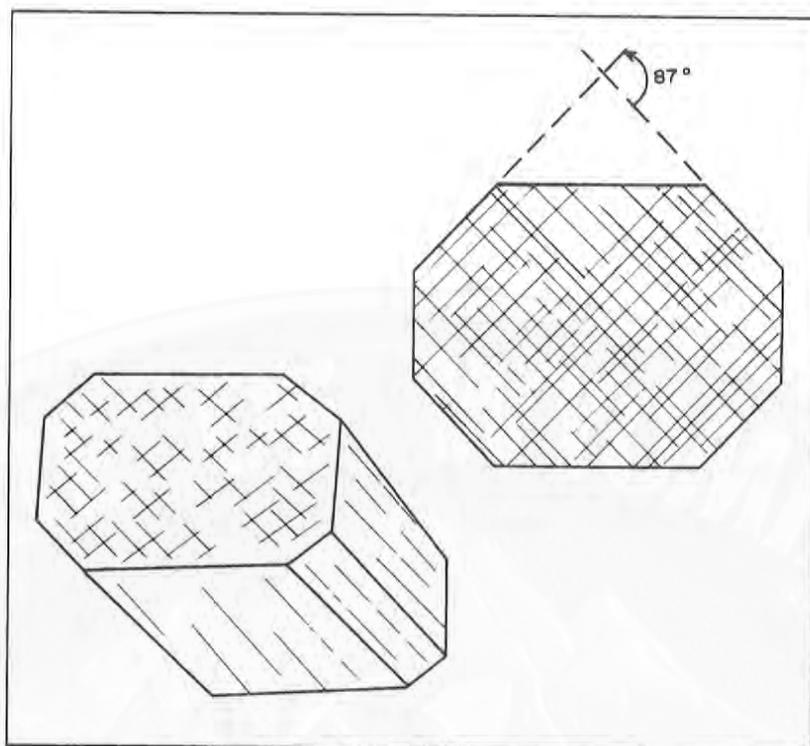
FIGURE 10—Typical pyroxene crystal showing major cleavages
