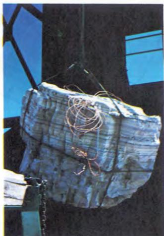
PLATE VIII-5 Block of oil shale being placed into United States Bureau of Mines experimental retort at Laramie
