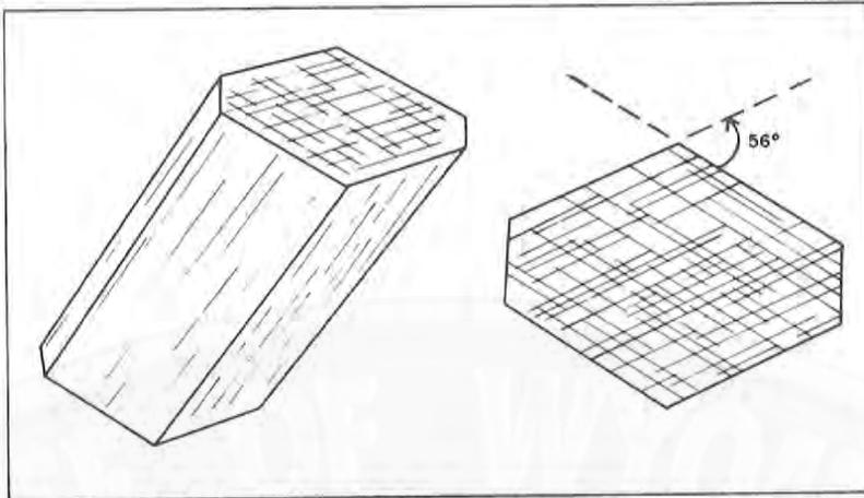
FIGURE 6—Typical amphibole crystal showing major cleavages
