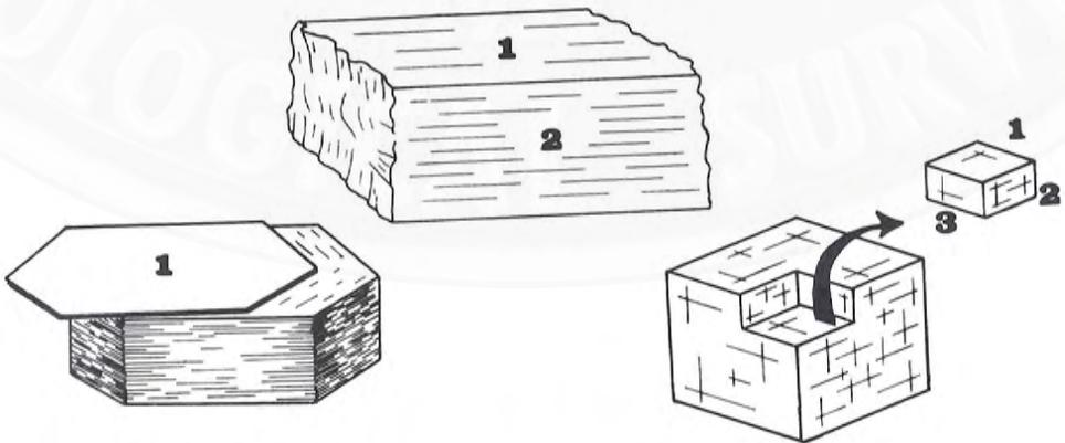
PLATE I-3 Cleavage in minerals; mica (left) has one prominent direction of cleavage, feldspar (center) has two and calcite (right) has three
