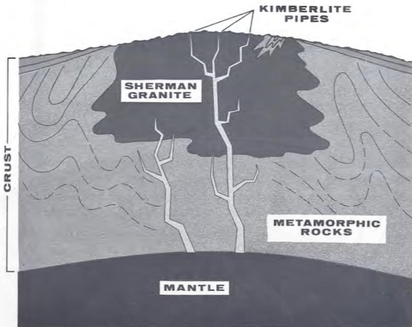
FIGURE 13—Diagram showing emplacement of kimberlite pipes
