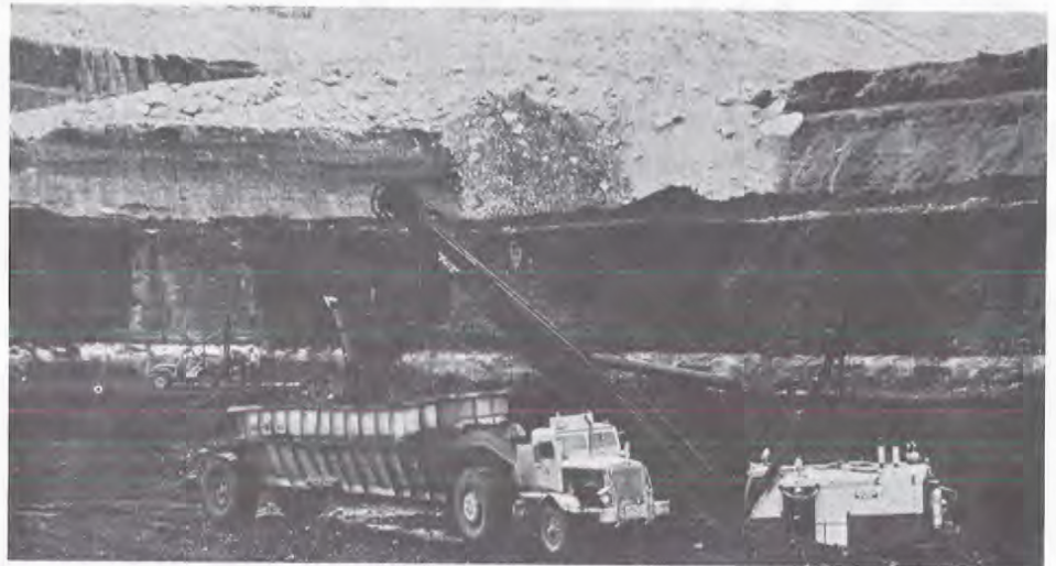
Big Horn No. 1 strip mine north of Sheridan, Wyo. Collectively the Monarch and Dietz coal beds are 44 feet thick at this mine. (Wyoming Geological Survey Photo)
