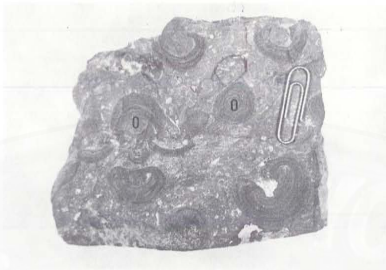
A. Photograph of Darby Formation (limestone sample from lower part). Unusual algal oncolites (O) in micritic matrix. Paper clip for scale is three cm long.
