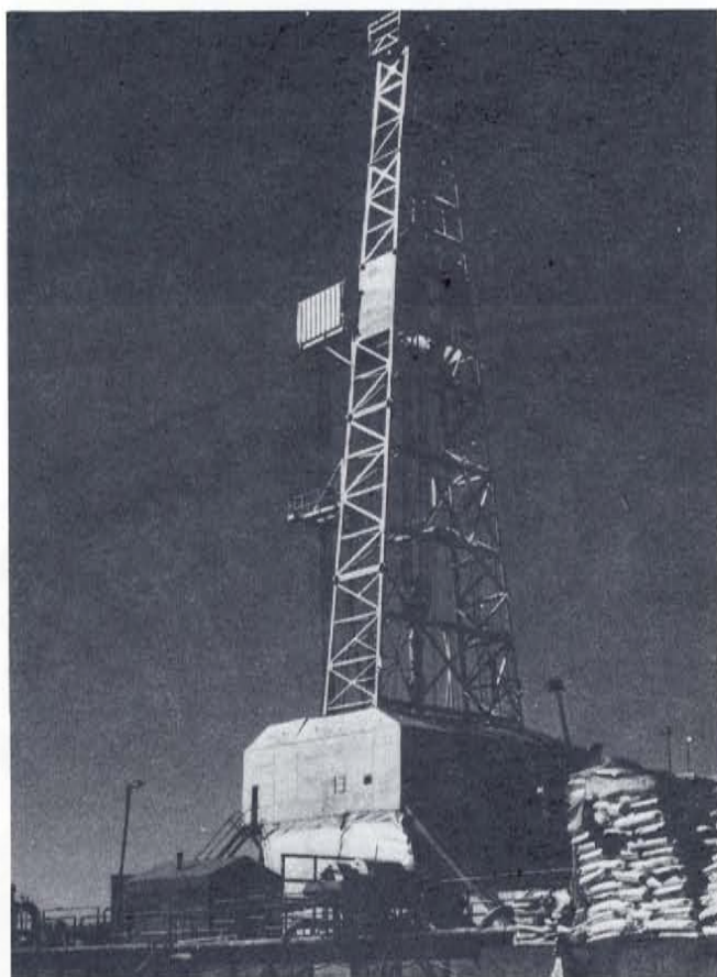
Figure 4. Parker Drilling Rig #112 contracted by Colorado Interstate Gas Company to drill the 1-6-36-86 Bullfrog Unit well in western Natrona County. This well was drilled to a depth of 20,850 feet in Waltman Field and completed in October 1979 in the Muddy, Dakota, Morrison, and Sundance, producing at the rate of 1,764,000 cubic feet of gas per day. (Photograph by compiler.)
