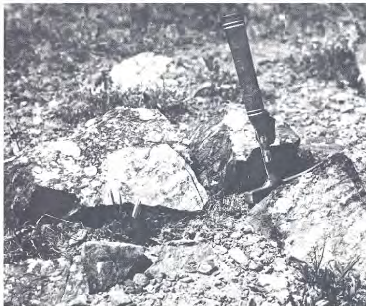
Figure 7: (a) Massive pyritized ore with colloform texture. This sample, collected in the Sierra Madres, exhibits rounded grains of pyrite mantled by chalcopyrite. The matrix is magnetite with minor chlorite. (b) Sierra Madre "Mill rock." Felsic volcanoclastics are often found in close proximity to massive ore. These felsic volcanic breccias are mapped in Canada and used as tracers to ore. Sangster (1973) dubbed these "mill rock" because whenever he was standing on a volcanoclastic with large fragments, he could hear the sound of a mill in the near background. Presumably, the volcanoclastics occur near minable ore and represent a fossil volcanic orifice from which the metallic sulfides originated. Photography by W. Dan Hausel, 1978.
