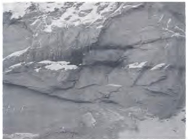
Figure 14: Exposed uranium roll-front in wall of Pathfinder Mines Corporation's Shirley Basin Mine. The roll-front forms the black concentric feature in the center of the photo. Photograph by W. Dan Hausel, 1977.
