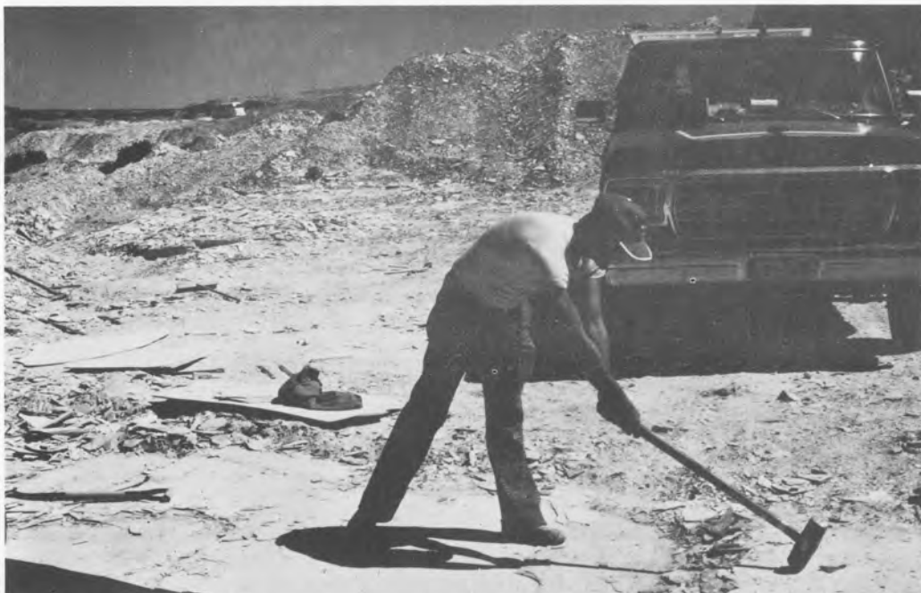
Figure AII.3. At F-1, the 3-5 inch, tough, dark-gray oil shale capping the 18-inch layer must be removed with hammers and shovels.
