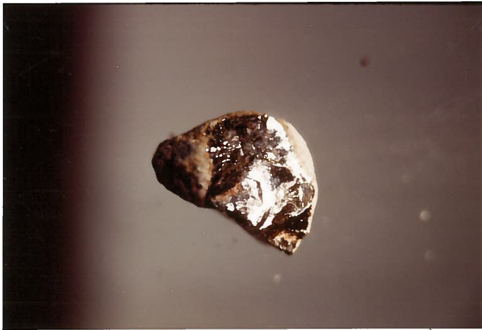
Figure 2. Picro-ilmenite megacryst from the Schaffer 15 pipe. Note the rounded nature, glossy black color on fresh surfaces, and remnants of leucoxene (a mixture of rutile and perovskite) coating. Grain dimensions are: 1 cm x 7.0 mm.
