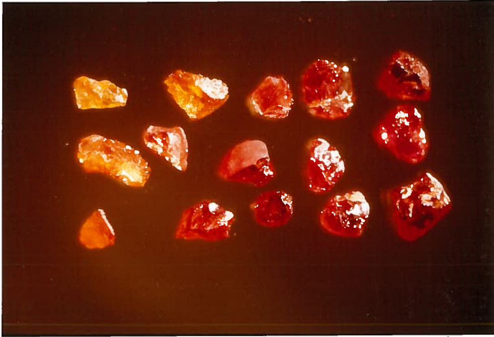
Figure 5. Fresh pyrope garnet grains from the Aultman 1 pipe. Color ranges from orange-yellow through red to deep red-purple. Note clarity (lack of inclusions) and remnant of original rounded surface on the center grain. Average grain size is 2.0 mm.
