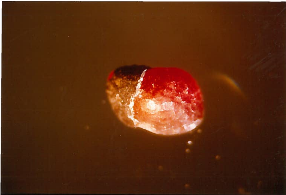
Figure 6. Pyrope garnet grain showing well-rounded nature caused by abrasion during kimberlite emplacement. The grain is partially covered by a rind of kelyphite formed by reaction of the garnet with the kimberlite matrix.
