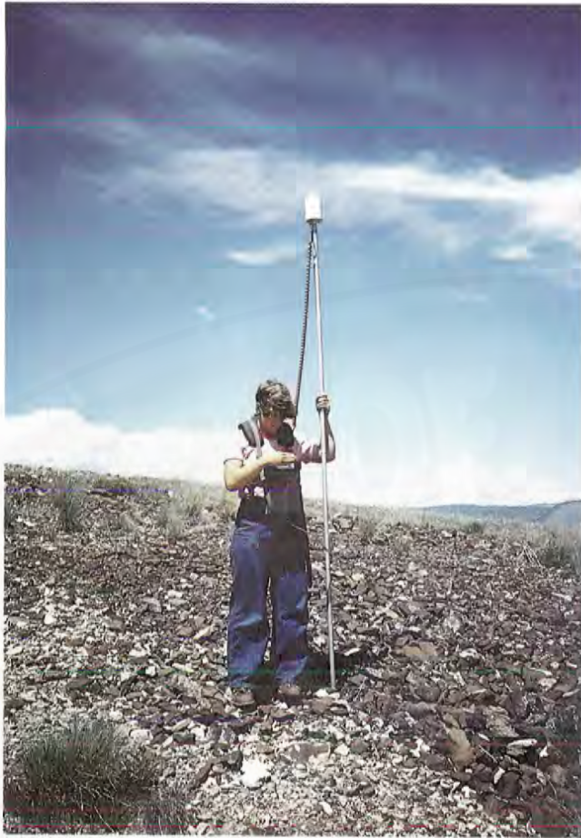
Figure 12: Outcrop of titaniferous black sandstone in the Mesaverde Formation about one mile south of the road. Photograph shows Wyoming Geological Survey geologist conducting magnetometer survey over the black sand. Because the black sandstones contain abundant magnetite, they are highly magnetic and susceptible to this kind of exploration technique (see Hausel and Jones, 1982). (Photo by W.D.H.)
