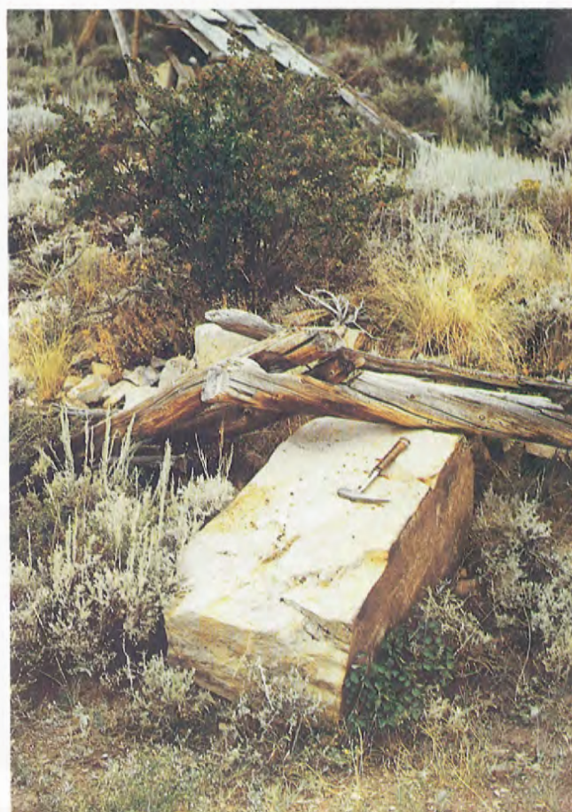
Figure 16: Large blocks of yellowish-brown sandstone like this one were quarried from the Cloverly Formation and used as building stone. (Photo by W.D.H.)
