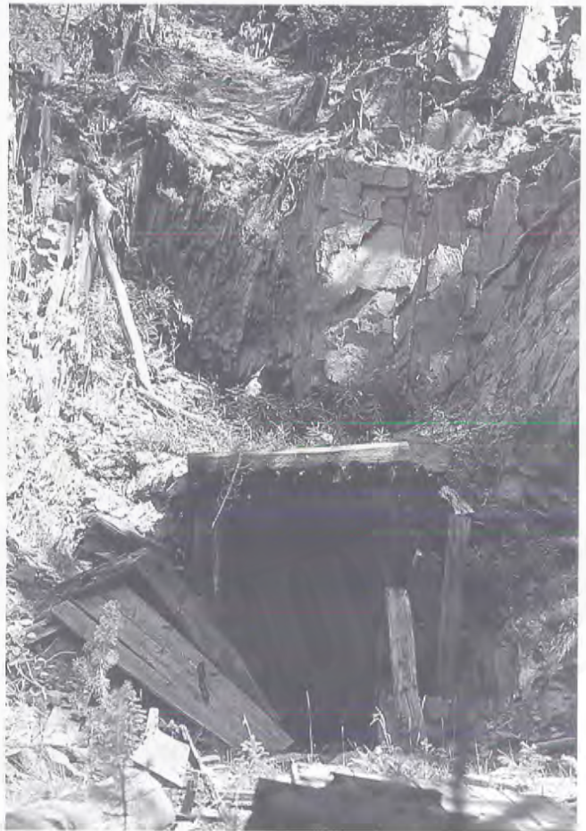
Figure 14: (B) An adit developed into sheared cataclastics along the Middle Fork of the Little Laramie River within the Centennial Ridge gold-platinum district. (Photo by W.D.H.)
