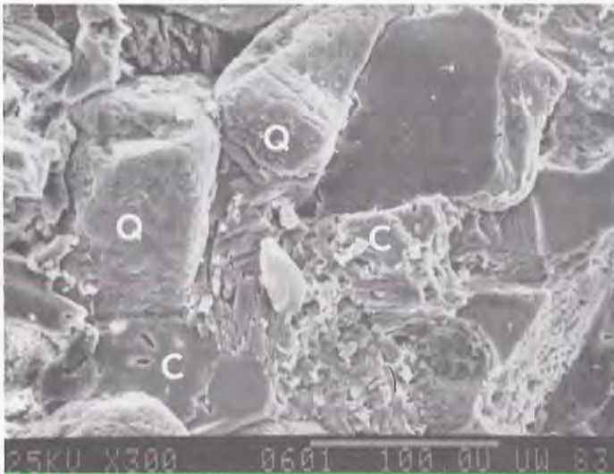
Figure 18B. Scanning electron micrograph of sample TCA-6-1, showing quartz grains (Q) cemented with calcite (C). This sample was collected from the basal barren zone. Magnification is 300X, and bar scale represents 100 microns.
