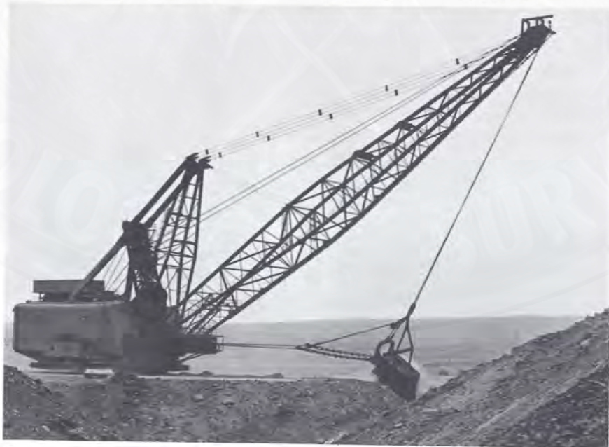
Dragline stripping overburden from coals in the newly rejuvenated Hanna coal field of southcentral Wyoming, 1972. (Photograph by G.B. Glass.)
