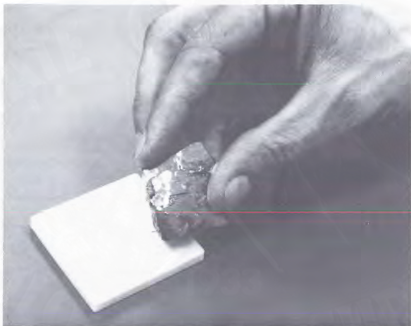
Figure 6. Scratching a streak plate with a galena cube produces a characteristic lead-gray streak (photograph by Karl Albert).
