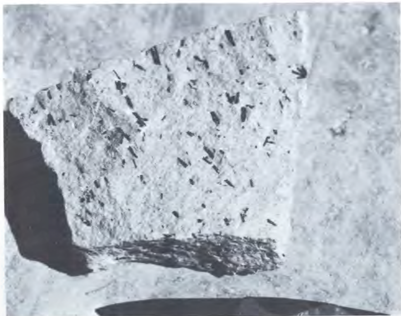
Figure 30. Andesite with large crystals (phenocrysts) of black amphibole enclosed by a light colored aphanitic groundmass, a typical texture of this igneous rock (photograph by Karl Albert).
