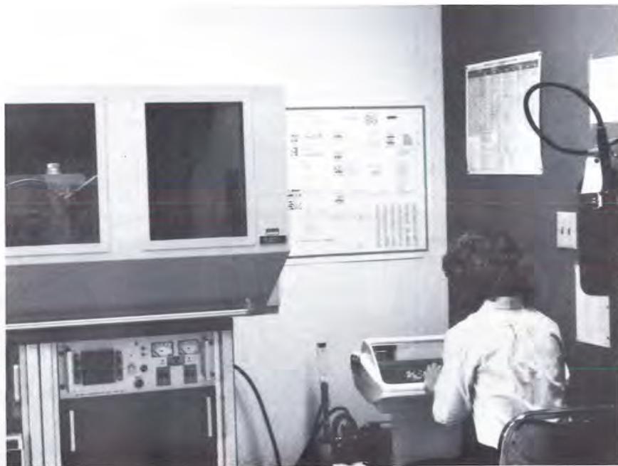
Figure 3. Mineral identification by specialized tests such as x-ray diffraction is common at many geological surveys, bureaus of mines and universities. At the Geological Survey of Wyoming, x-ray analysis is carried out with a state-of-the-art computerized diffractometer (photograph by Karl Albert).
