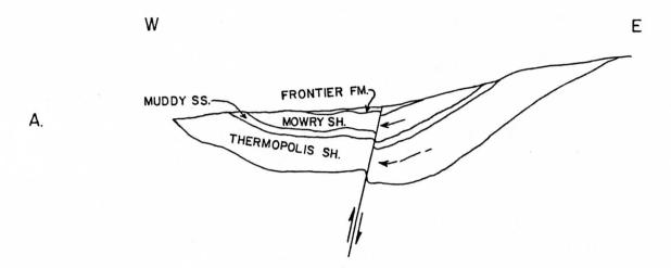
Inferred flow of ground water with reverse fault present as indicated on Geomax cross section.
