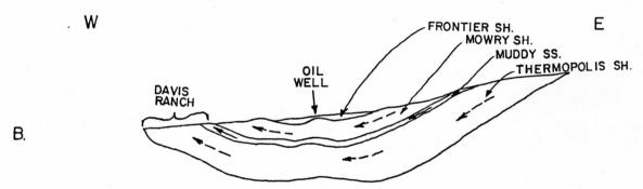
Inferred flow of ground water with reverse fault not present.
