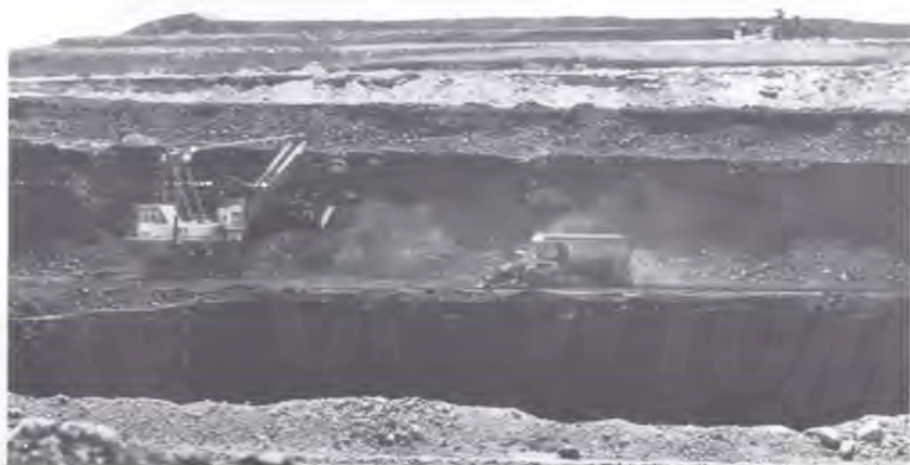
Figure 52. At this large surface coal mine north of Gillette, miners are stripping the upper half of a coal seam over 110 feet thick. The coal shovel (left) is 50 feet high and has a 40-cubic-yard bucket. The coal haul truck (center) handles about 120 tons (150 cubic yards) of coal. (Photograph by Richard W. Jones.)
