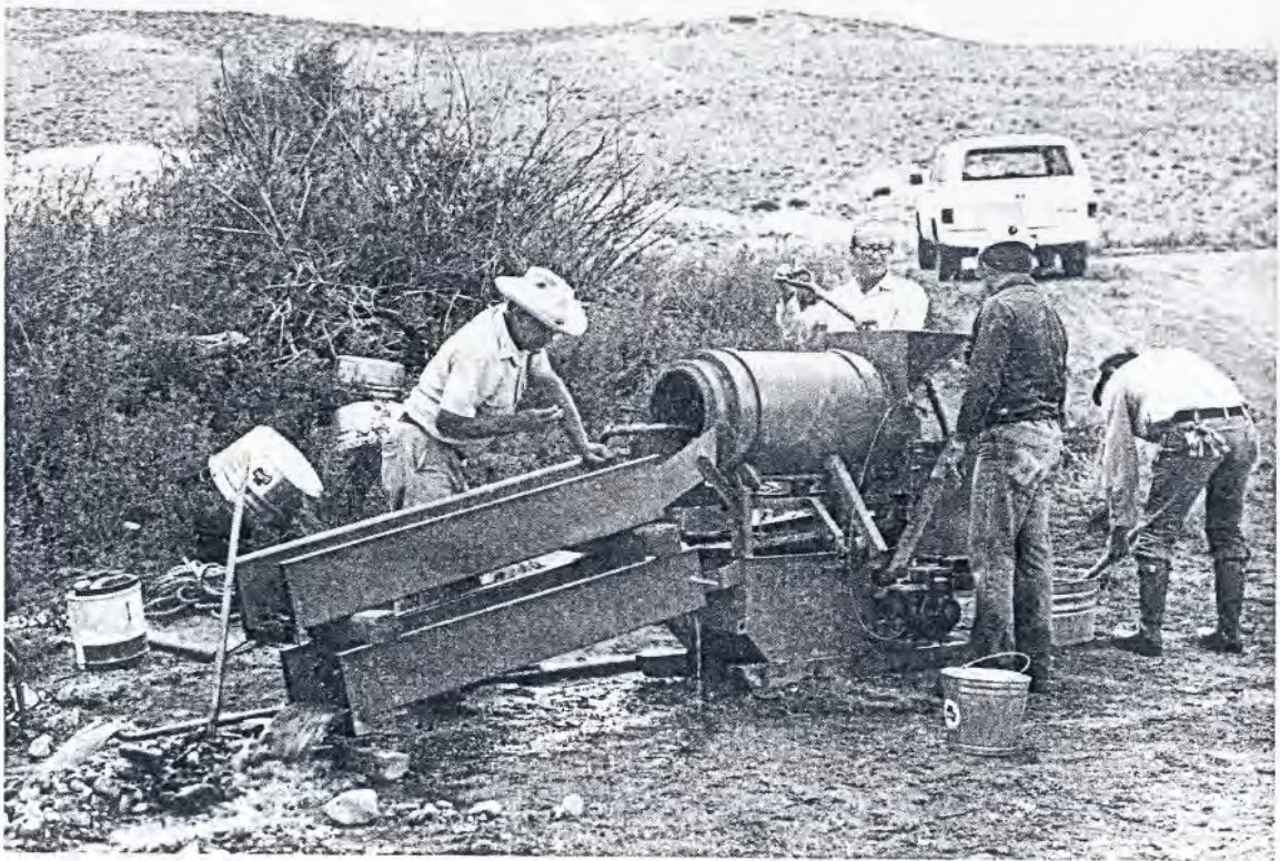
FIGURE 10.—Mechanical concentrator being used to obtain heavy sand concentrates from gravel samples.
