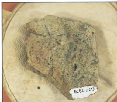
Plate 2B. The stockworks in the Eagle Creek district include intensely phyllically altered (bleached) latite with abundant pyrite.
