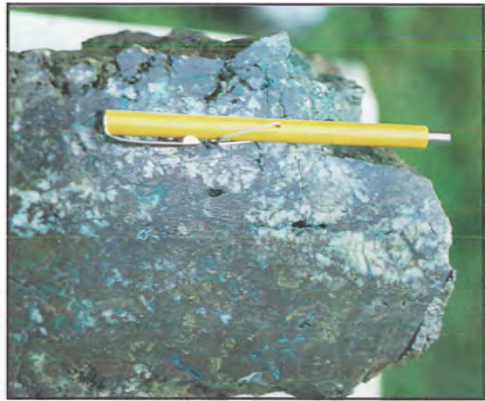
Plate 3B. Massive chalcocite-cuprite-chalcopyrite with minor malachite and chrysocolla filling fracture in milky quartz vein from the Kurtz-Chatterton mine, Encampment district.
