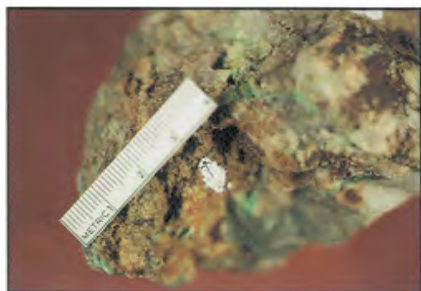
Plate 4A. Copper-stained limonitic quartz from the Penn mine area, Seminoe Mountains. Arrow points at small rod of visible gold.
