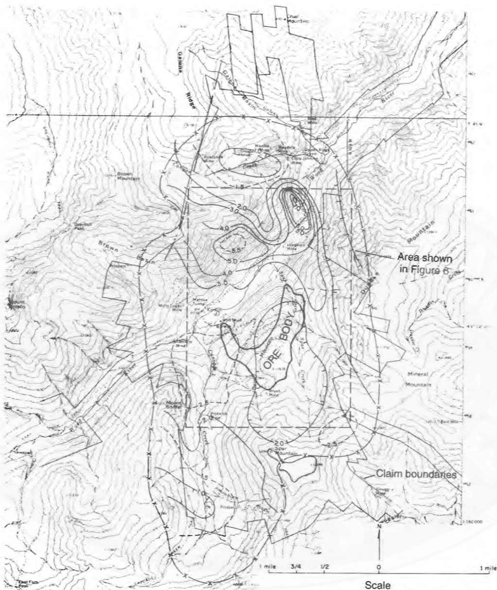
Figure 7. Aeromagnetic map over the Kirwin mineralized area, Park County, Wyoming. The prominent magnetic high north of Kirwin is interpreted to be a response to a buried, high-grade skarn (modified from AMAX Exploration Inc. map, Wyoming State Geological Survey files). Terrain clearance = 1000 feet approximate. Contours are \times 100 gammas; x'ed line indicates outline of area surveyed.
