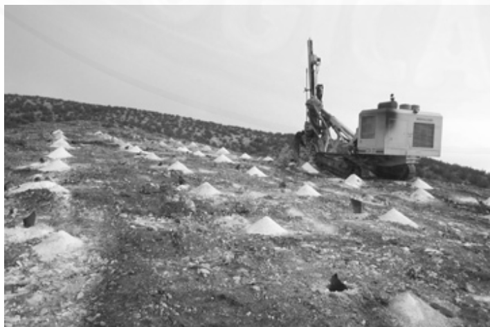
Figure 22. Reserve drilling by Slate Creek Stone at the Grant Ranch marble quarry site, Platte County, Wyoming, September, 2000.
