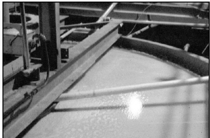
Figure 28. Yellowcake in vat at CAMECO's recovery plant. This material will be dried and shipped in airtight containers. This material poses no radiation threat to the photographer or the plant workers, since pure uranium emits only alpha particles, which do not penetrate the skin or clothing. The only radiation safety equipment needed is a respirator.
