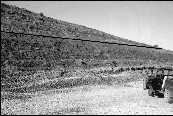
Figure 21. The Clay Spur bentonite bed (between the vehicle and the black line) contains a major bentonite resource in the Colony mining district, Crook County.
