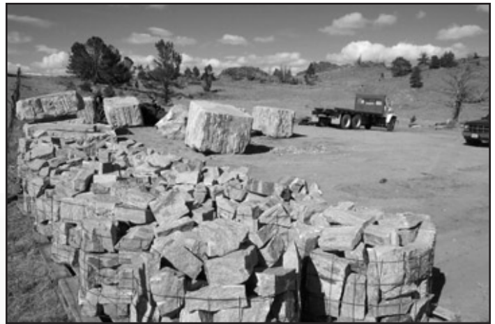
Figure 18. Dimensional stone (blocks and split-face fieldstone) at the quarry site operated by Raven Quarries in northern Albany County, Wyoming.
