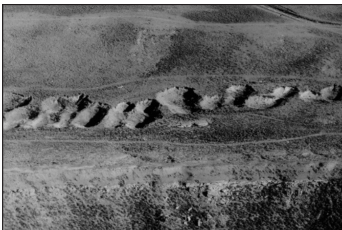
Figure 28. Oblique air photograph of surface subsidence features over abandoned underground coal mines near Hanna. Photograph by Gary B. Glass.
