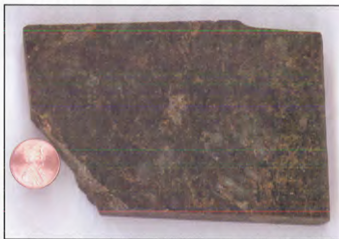
Figure 34. Polished sample of dark syenite, typical of that found in any of the four Sybill Canyon quarry sites.
