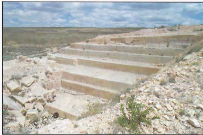
Figure 50. The quarry face at the University of Wyoming's Casper sandstone quarry. Each lift is about 6 feet high.
