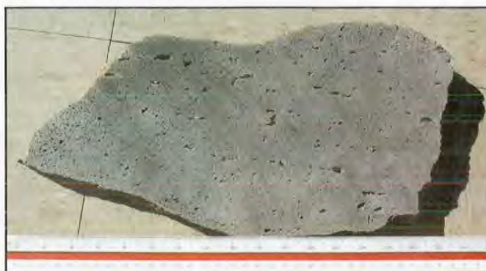
Figure 124. Cut sample of basalt from Horse Mountain area; engineering scale is about 1 foot long.
