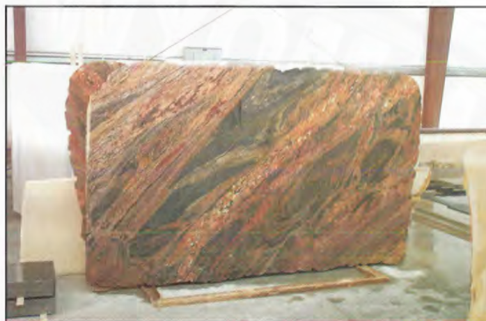
Figure 8. Polished slab of Mirage® from Raven Quarries, LLC. This slab is 5 feet high, 10 feet long, and 5/8 inch thick.
