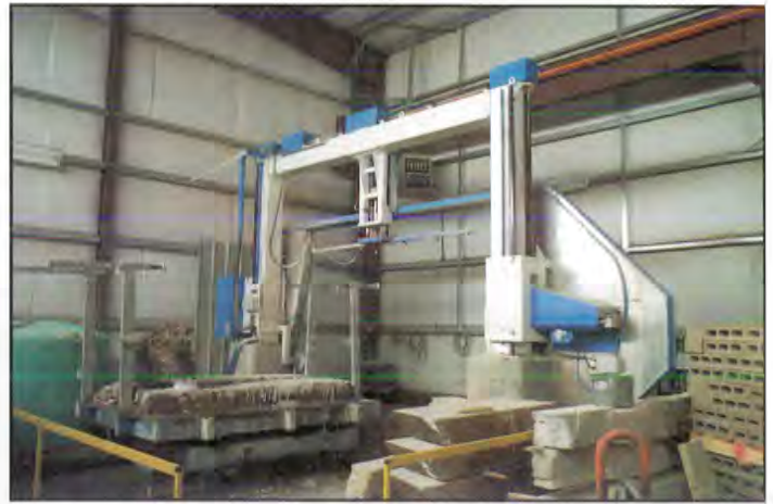
Figure 1. Wireline saw used at Strid Marble and Granite's fabricating plant in Cheyenne. Note movable trolley. Height of this saw is about 15 feet.
