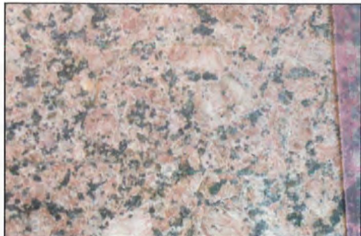
Figure 61. Polished sample of pink granite from the No Name Rock site. Scale is inches. Field of view is about 5 inches wide and 4 inches high.
