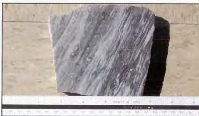
Figure 23. Polished sample of Bluegrass marble. Upper scale is inches, lower scale is centimeters.
