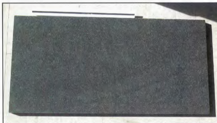
Figure 6. Polished 24 inch by 12 inch "slab" of Wyoming Raven®. Engineering scale is about 12 inches long.
