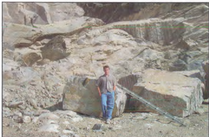
Figure 7. Formerly active quarry for Mirage® granite. These blocks were cut into slab and polished.
