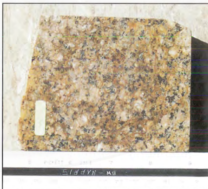
Figure 29. Polished sample of Red Mountain granite. Upper scale is inches, lower scale is centimeters.
