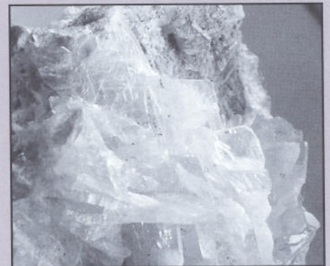
Figure 22. Cleavage displayed in specimen of barite from Transylvania. Note the individual crystals in the center of the photo are flattened plates with c[001] axis perpendicular to this page. These flat surfaces also represent the basal cleavage. At right angles to the c-axis are flat edges that are nearly perpendicular to one another. These crystal faces represent prismatic cleavage at right angles to the c-axis.
