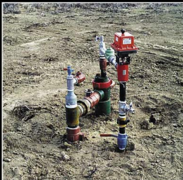
Figure 8. Typical coalbed methane wellhead in the Powder River Coal Field with water and gas lines installed and a control box (red) in place. Photograph from Wyoming Coalbed Methane Clearinghouse web site, 2004.
