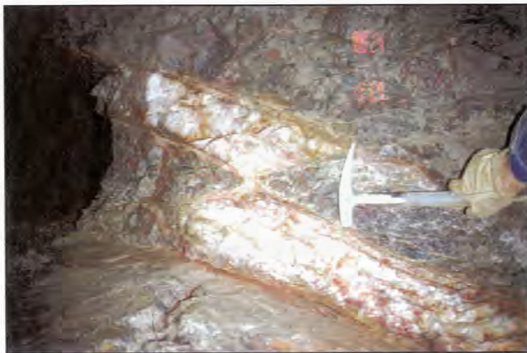
Figure 6. Faulted quartz vein exposed in the Mary Ellen gold mine at South Pass.
