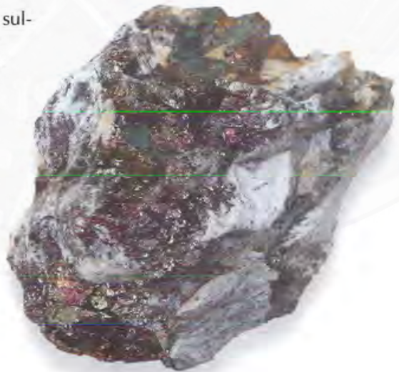
Figure 32. Bornite specimen from the Ferris-Haggarty mine in the Encampment district of the Sierra Madre. Distinct multi-colored bornite found with green malachite, bronze, metallic pyrite, and chalcopyrite all in deformed metaconglomerate.
