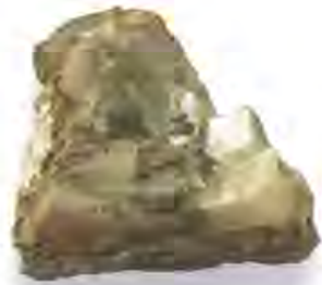
Figure 34. Calcite rhombohedral crystals with minor chlorite and polybasite from Cooper Hill, Medicine Bow Mountains. Note the distinctive calcite rhombohedrons reflecting light near the center of the photo.
