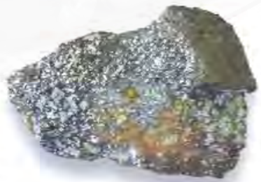
Figure 64. (a) Cumulate textured, black magnetite in serpentinite from Lake Owen area, Medicine Bow Mountains.
