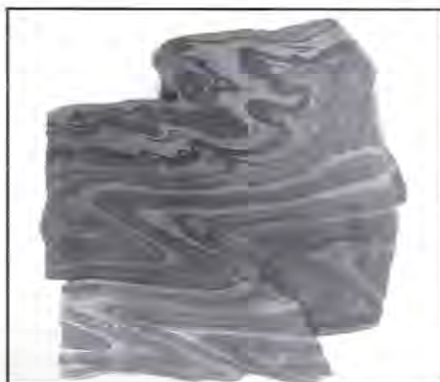
Figure 64. (b) Typical banding in isoclinally folded taconite showing alternating layers of chert and magnetite.
