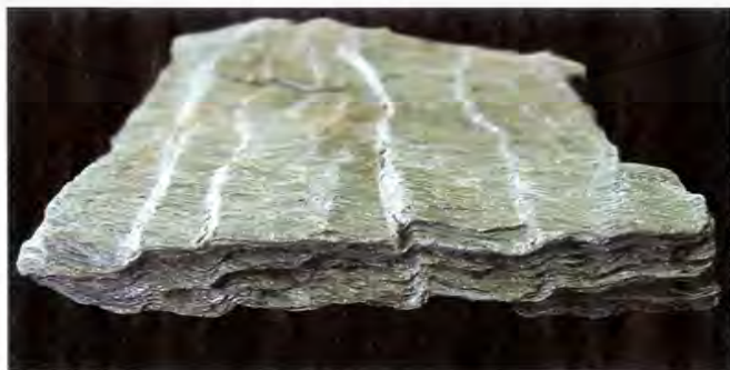
Figure 91. Chlorite-talc-actinolite schist showing distinct schistose layering. Sample from the Carrissa mine, South Pass.
