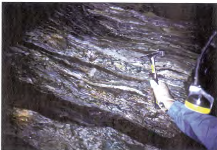
Figure 33. Copper ore from the Ferris-Haggarty mine, Sierra Madre. Massive malachite, bornite, chalcocite, covellite, and chalcopyrite form the matrix of Precambrian metaconglomerate.
