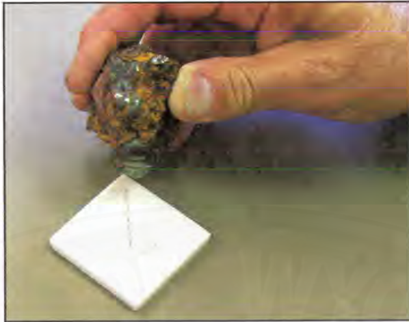
Figure 16. Scratch test on a streak plate tile with hematite which produces a distinctive red streak.
