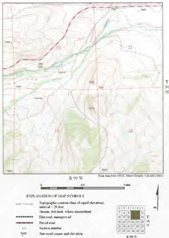
Figure 109. A part of the U.S. Geological Survey Miners Delight topographic map. Township 30 North (T30N) is labeled in the right margin and Range 99 West (R99W) in the lower margin. Sections are numbered and a portion of section 11 occurs at the upper right. The southwest quarter is the lower left hand portion of section 11.
