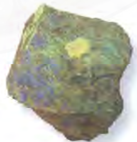
Figure 29. Blue azurite with green malachite stains this schist from the American mine, Medicine Bow Mountains.
