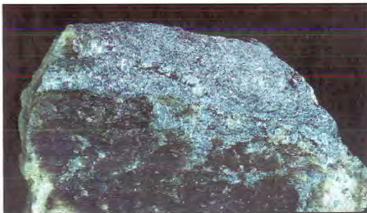
Figure 27. Tiny acicular prismatic metallic crystals of arsenopyrite scattered in massive arsenopyrite with limonite and scorodite (yellow) and hematite (dark red). Specimen collected near Garrett, Wyoming.
