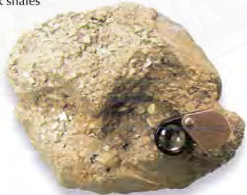
Figure 73. Pyrite cubes in quartz from the Lost Muffler mine, Rattlesnake Hills. Note the distinctive bronze metallic luster and crystal habit.
