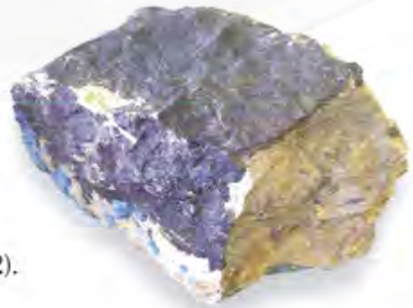
Figure 82. Tenorite (black) with azurite (blue) and altered sandstone from the Griggs mine, Lake Alice district, western Wyoming.
