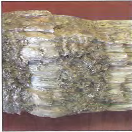
Figure 81. Talc (fibrous) veins in chlorite schist from Tin Cup district, Granite Mountains.
