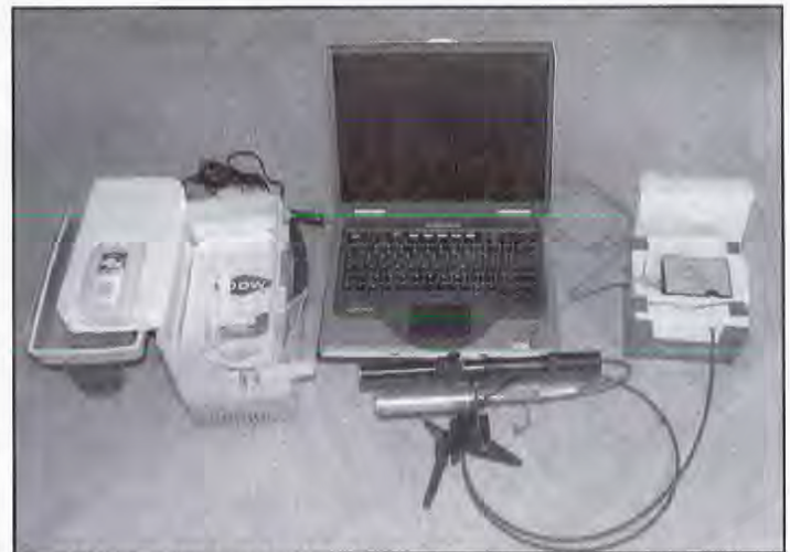
Figure 1. Computer, spectrometer, cooling options, and collector head.
