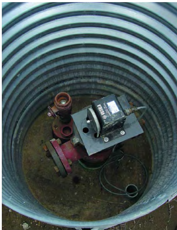
Figure 4. Counter balance tape used for deep well measurements. Photo by Richard Hays.
