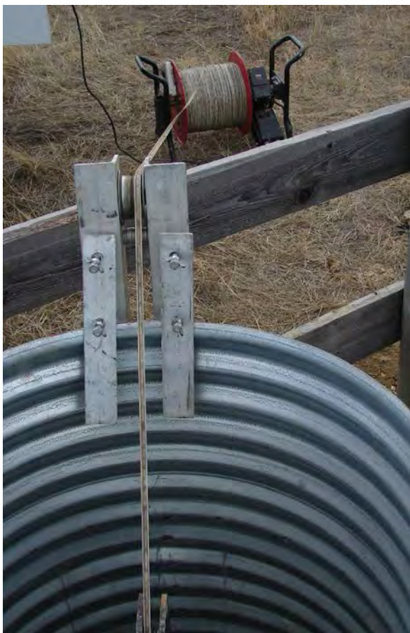
Figure 3. Electronic tape measuring system in use at the Juniper monitor well site location. Photo by Richard Hays.
