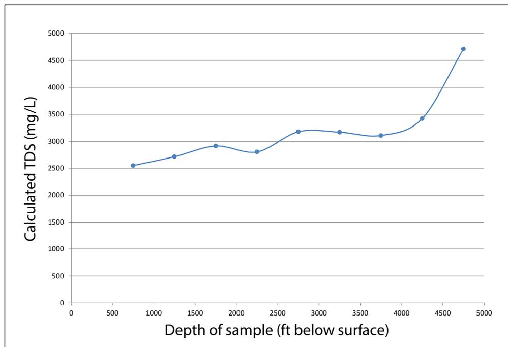
**Figure 3.** Mean calculated TDS levels versus depth of sample.
