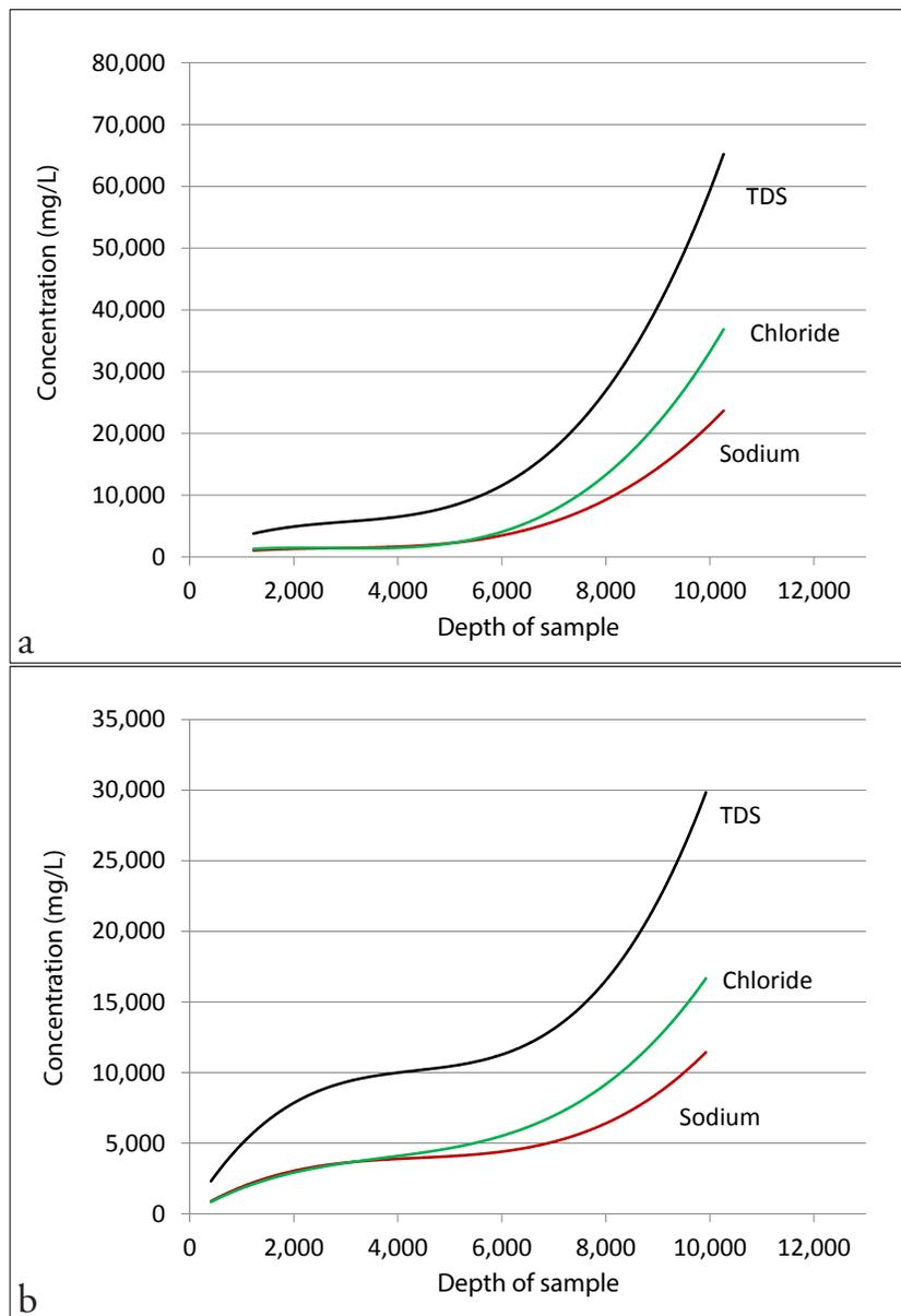
**Figure 1.** Trends in TDS, sodium and chloride levels with depth of sample in the a) Casper-Tensleep Formation of the Laramie Basin, and b) Newcastle Sandstone of the Powder River Basin, Wyoming.
