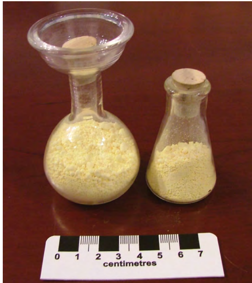
Figure 17. Yellowcake ( \text{U}_3\text{O}_8 ), the end product of uranium mining. (Photo courtesy of Strathmore Minerals, Riverton, Wyoming, 2010).
