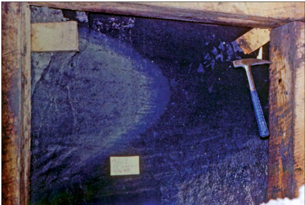
Figure 4. Underground mine photo of a well formed roll front with associated high grade uranium ore on the right side of the front (Photo courtesy of R.V. Bailey, circa 1960).
