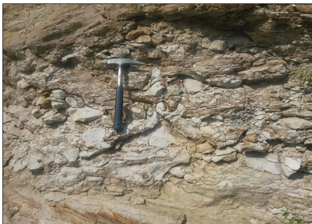
Figure 63. White tuff of the upper part of the lower sequence rocks of Lysite Mountain (Bay, 1969). This unit hosts a minor amount of clinoptilolite and heulandite (Sample 20150820DB-2).
