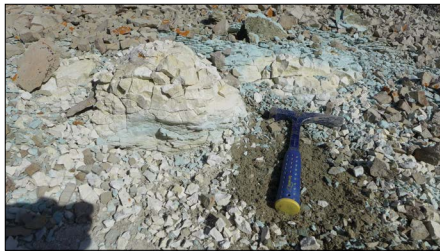
Figure 21. Outcrops of robin's-egg-blue tuff showing the subtle difference between the blocky buff and generally platy blue zeolitic tuff beds in the W1/2 section 12, T. 16 N., R. 98 W., Sweetwater County.
