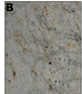
Figure 24. A) Zeolitic tuff (Sample 20141106BG-3) collected from the lower part of the Adobe Town Member near Eagle Nest Draw in SE1/4 SW1/4 sec. 28, T. 16 N., R. 98 W. B) Close-up showing scattered biotite laths and iron oxide staining.
