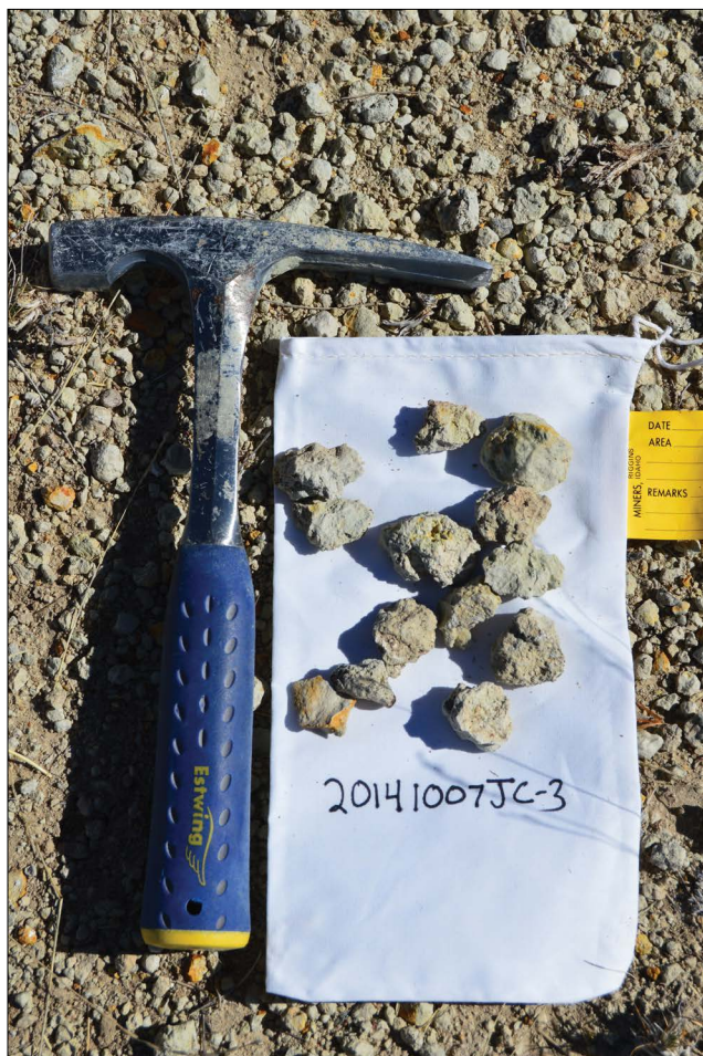
Figure 68. Sample 20141007JC-3. Gray to yellowish-brown, limonite stained mudstone. No outcrop is present at the sample location, but pebbles of this mudstone cover the ground. This mudstone hosts minor amounts of mor-denite.
