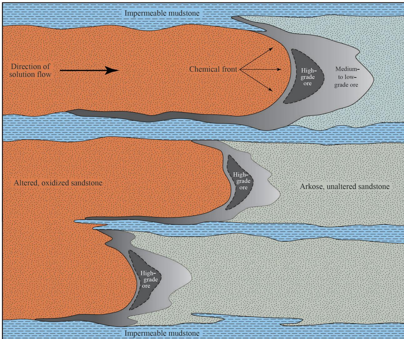
**Figure 13.** Cross-sectional depiction of an en echelon arrangement of a series of roll-front uranium deposits. Modified from Nielsen, 2013.
