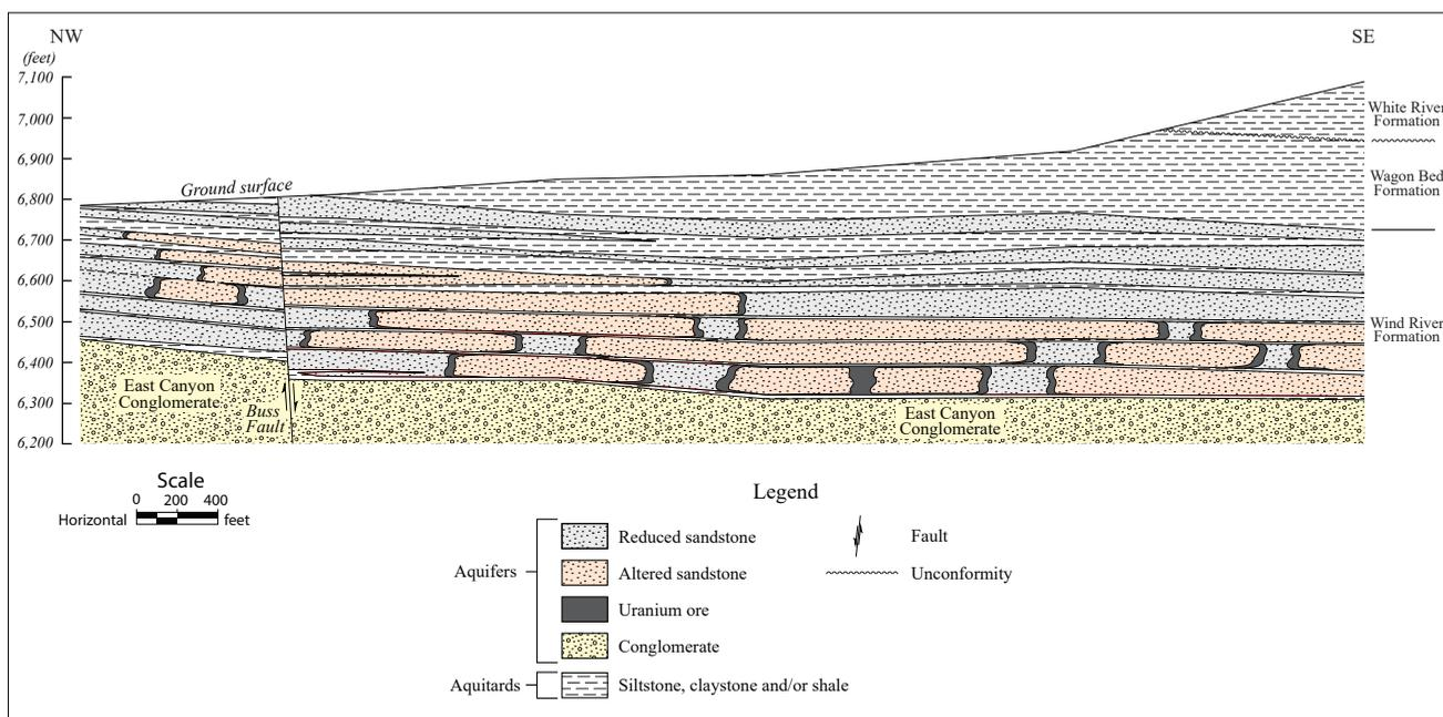
**Figure 14.** Cross-sectional view of an echelon stacking of roll-front deposits in the Puddle Springs Arkose Member of the Wind River Formation in the eastern Gas Hills. Modified from Power Resources Inc., (1996). As uranium-bearing fluids infiltrate the fan system, the migration of a given roll-front will fan out similar to the development of the original fan system, resulting in some instances of roll-fronts migrating toward each other (bottom ore horizon).
