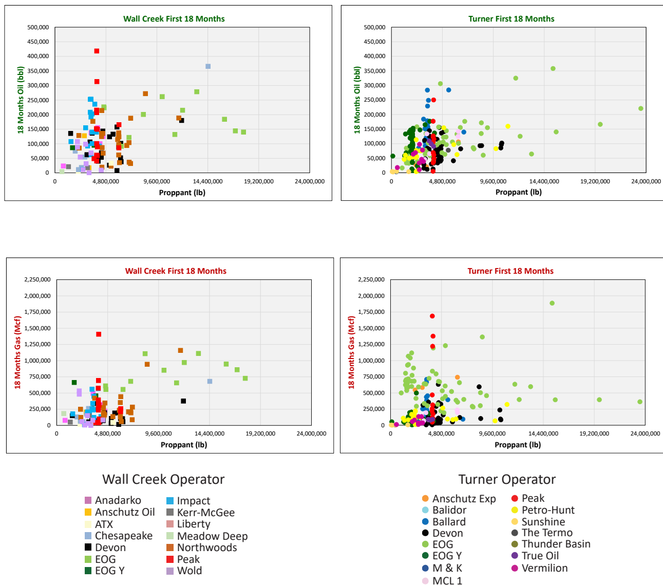
Figure 16. Amount of proppant used in horizontal well completion versus first 18 months of unconventional oil (top row) and gas (bottom row) production. Wall Creek wells are in the left column and symbolized by squares; Turner wells are in the right column and symbolized by circles. Wells are colored by operator. Operators not displayed on graphs do not have wells with 18 months of production.
