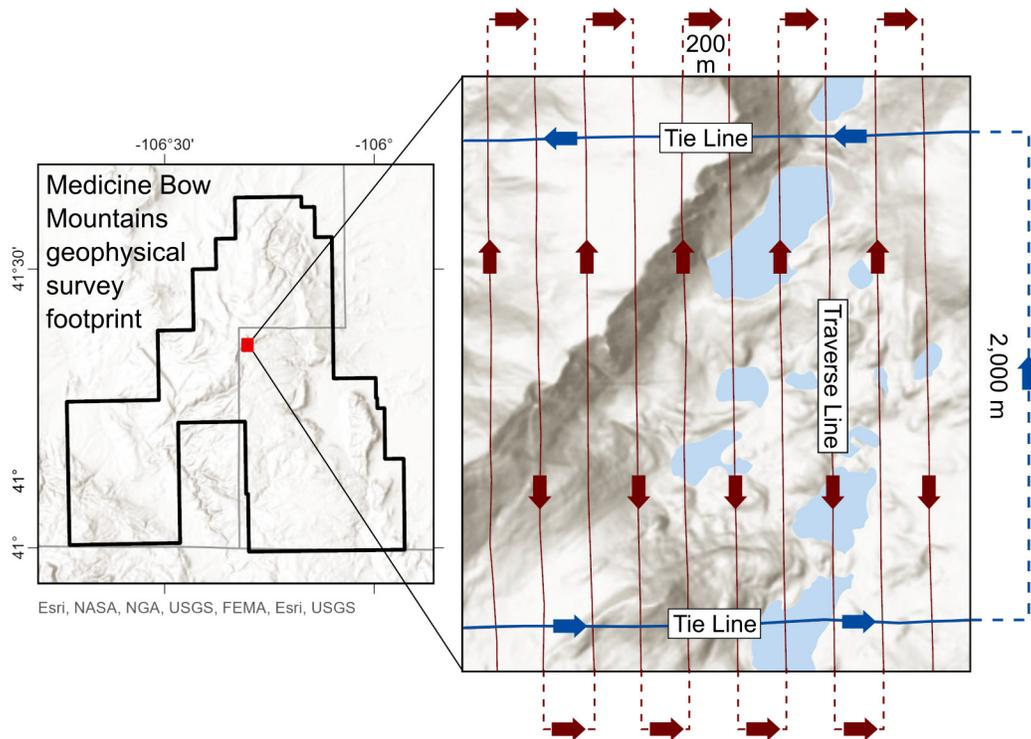
**Figure 4.** Map showing an example of traverse lines and tie lines from the Medicine Bow Mountains geophysical survey, focusing on the Snowy Range area. Dashed lines are for illustrative purposes only and do not show the full extent of the flight lines. Basemap: Esri (2005).
