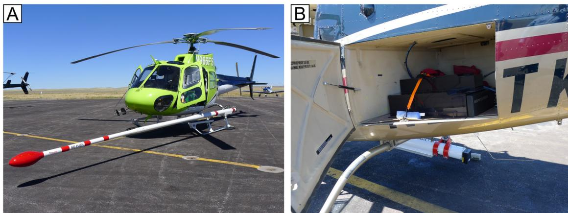
**Figure 3.** A) Helicopter with stinger-shaped magnetometer (white with red tip). B) Gamma ray spectrometer (black boxes) mounted inside a helicopter.
